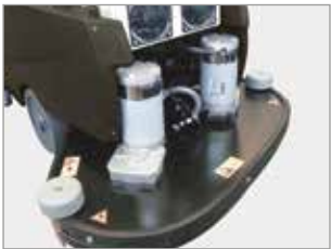
BRUSH HEAD SETTABLE BY ACTUATOR
