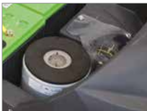
THREE-PHASE VACUUM MOTOR
