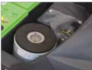
THREE-PHASE VACUUM MOTOR
